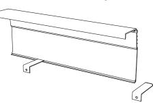
6. Position new assembled cover with wall brackets below element, then slip new cover over back panel.
