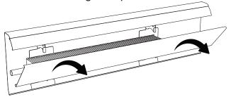
3. Remove any existing damper sections.
